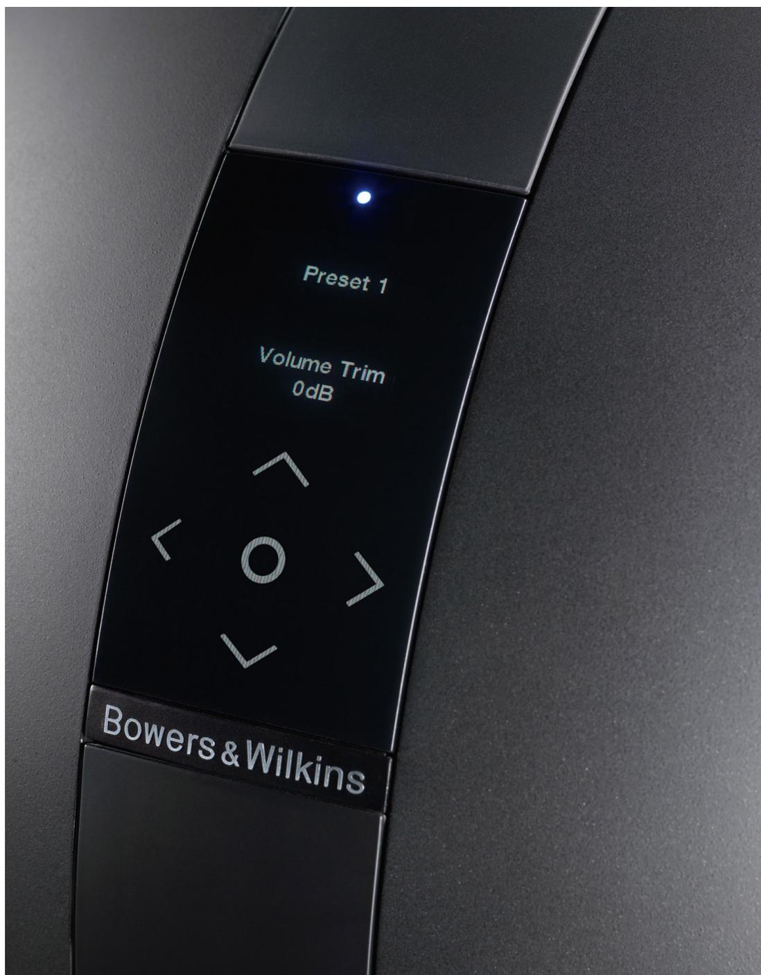
The display indicates which Preset is in play and a parameter called Volume Trim. This is an extra gain over and above the global configuration that allows the user to adjust the PV1D's level on the fly for individual programme items. Below this information are the navigation touch buttons. The display fades after 30 seconds of non-use and is reactivated simply by touching the button area.
