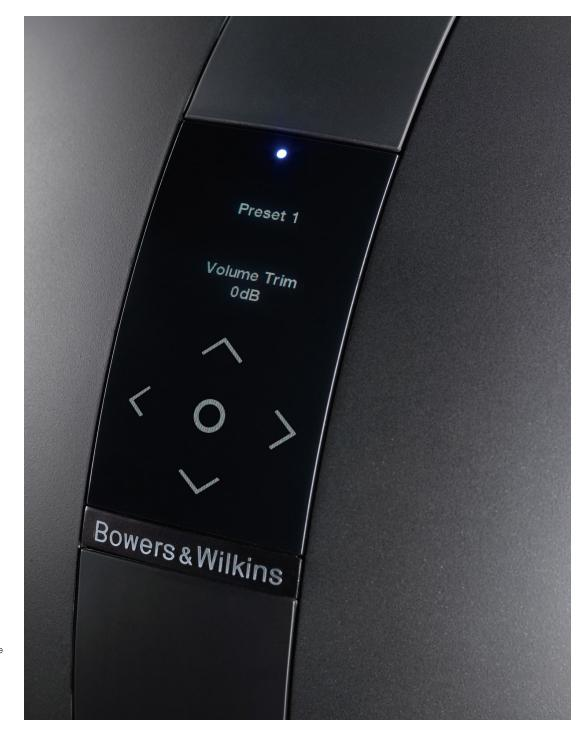
The display indicates which Preset is in play and a parameter called Volume Trim. This is an extra gain over and above the global configuration that allows the user to adjust the PV1D's level on the fly for individual programme items. Below this information are the navigation touch buttons. The display fades after 30 seconds of non-use and is reactivated simply by touching the button area.
