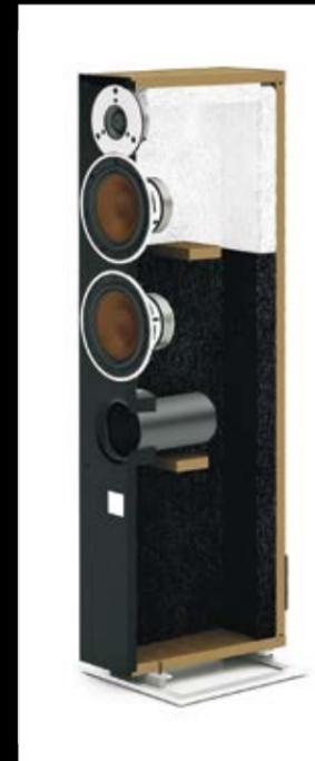
**Cabinet** | CNC machined MDF board, dressed in a top-of-the-class laminate forms the framework of the speaker. In addition, the floor-standing models feature strong internal bracing to reduce structural resonances.
